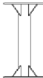
Optional Floor Mounted Pedestal Stand
